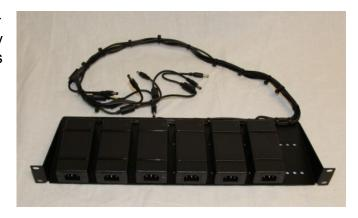
The next power supply will power the blade to the far right of the chassis (as viewed from the fan box opening). There will be one additional power supply included in the shipment. This power supply is for the chassis to provide power to the cooling fans. Dressing the DC power leads as shown will keep the DC power wiring neat and out of the way.
