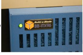
During normal operation the fan alarm will be silent and the green LED on the front panel will be on steady as shown at right.
